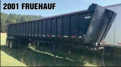
2001 FRUEHAUF Frameless Steel End Dump, 39 Ft. Long, 102 Inches Wide, Steel Frame, Swing Gate, Air Ride Suspension, 11R22.5 Disc Wheels
